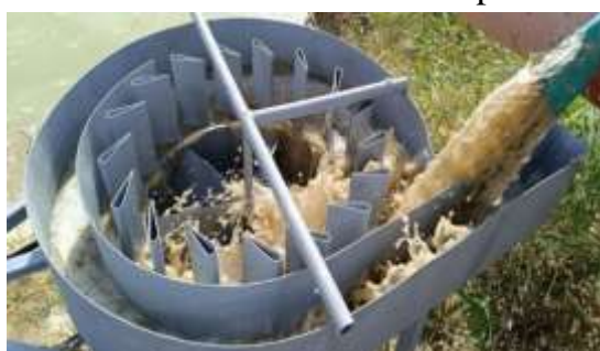
Fig. 2. - Experimental installation of a microelectric power plant with a vertical axis
