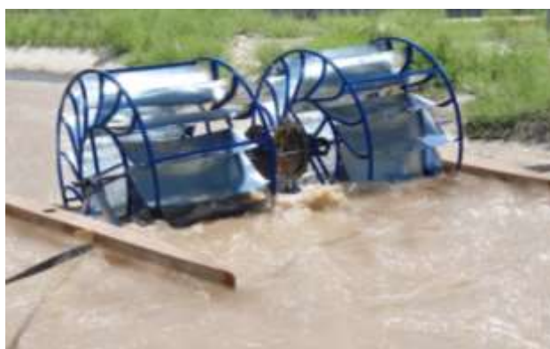
Fig. 3. Conducting an experiment of a developed micro hydropower plant
