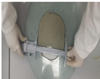
Figure 2. Determination of the optimal dosage of the chemical admixture “Sika 43-36” using the mini-slump test
