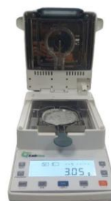
Figure 1. Determination of the concentration of the chemical admixture using a moisture analyzer
