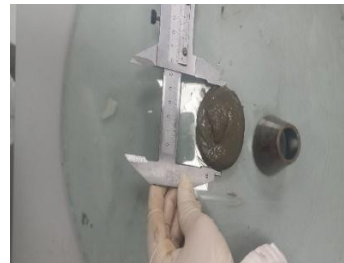
Figure 2. Determination of the optimal dosage of the chemical admixture “Sika 43-36” using the mini-slump test
