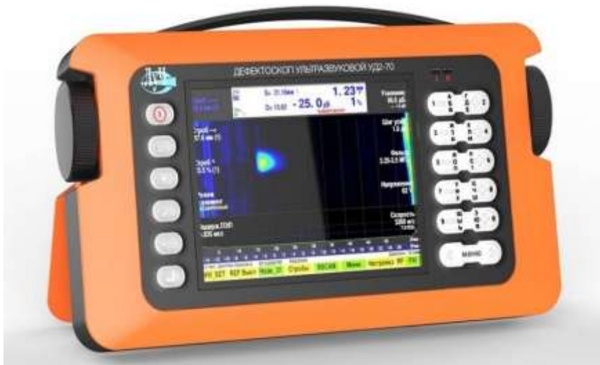
2-rasm. UD2-70 ultratovushli nuqson detektori
